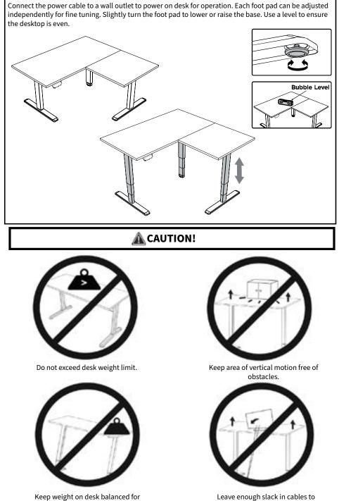
Leave enough slack in cables to allow for full range of vertical motion.
